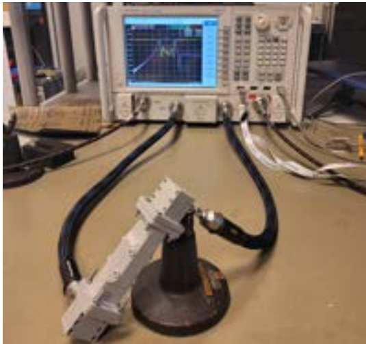
FIGURE 13. Measurement setup using WR-75 waveguide-to-coax adapters.
