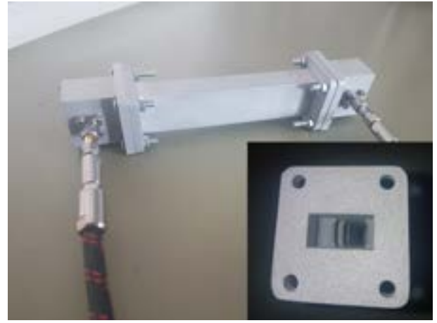
Fig. 4. A 3D-printed prototype of the filter.
